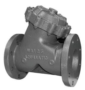
The Y-pattern diaphragm valve, with large seat opening and high lift disc, permits greater flows at lower pressure loss than any comparable valve. Positive control action is achieved, either hydraulically or pneumatically without the aid of springs. Components are serviceable while the valve is in line. These valves are available in both metallic and thermoplastic materials and are ideal for water treatment equipment such as water softeners and media filters.
